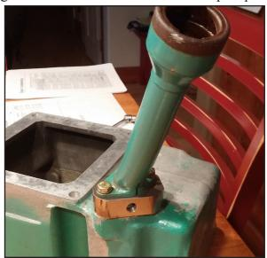
The oil sump return looked like this less the oil return barb. The barb fitting was put in after the engine was installed in the motorcar.... not wanting to have it broken off during installation.
