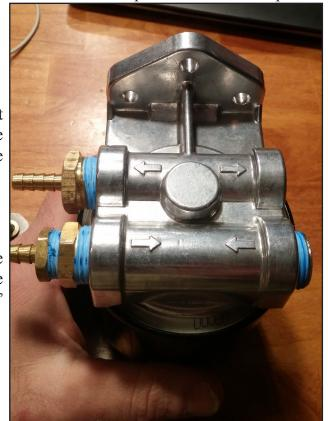
The top right outlet port gets a 1/2" NPT x 1/8" NPT reducer bushing. The oil flow restrictor then threads into the bushing and then a 1/8" NPT x 1/4" hose barb into that.
